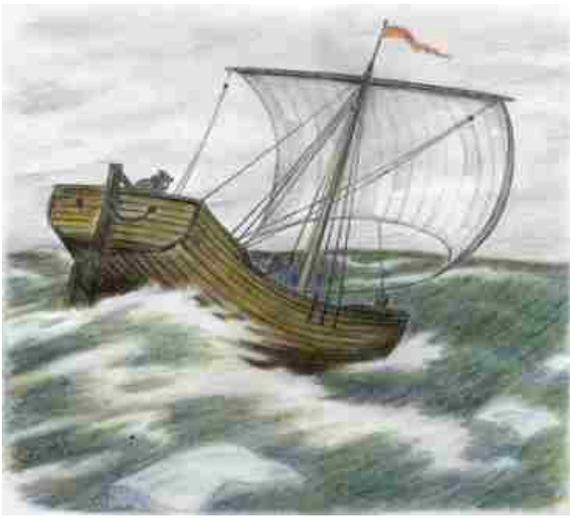
**Following Sea.** Fishing vessel of the Russian pomors (coast dwellers known for daring arctic voyages at the time of the Vikings). The hull form allows active maneuvering in gale seas with the storm sail and drag to stern allowing the vessel to run in a following sea. [http://www.science.sakhalin.ru/Ship/Vlad\\_R1.html#p3](http://www.science.sakhalin.ru/Ship/Vlad_R1.html#p3) Used with permission [2]
